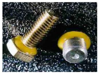
The surface finish of the mating surfaces should ideally be Ra3.2 and there should be no sharp edges on either surface as this could adversely affect the sealing capability of the Hyloseal. When a suitable lubricant is added as a final finish, the products can be re-used up to 12 times.
